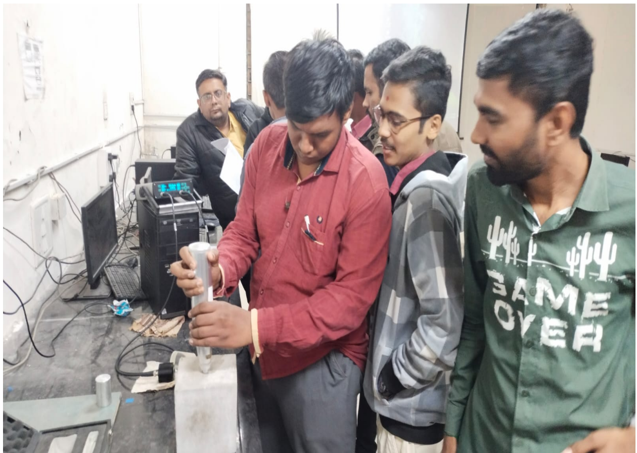
DEMOSTRATION& HANDS ON PRACTICE OF ULTRASONIC MACHINE& REBOUND HAMMER
